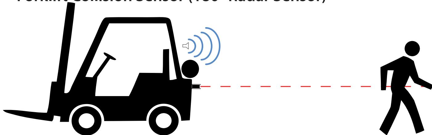
Frequency of LED increases as sensor draws closer to obstruction
